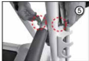
3: lift up the armrest of electronic watch and use two M8\*50 screw through armrest hole to the stand pipe, then screwed tightly (don't press the signal lines). Then cover the armrest guards in the armrest.
